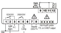
12Vac/dc supply: connect to the terminals 7 and 8. 24Vac/dc supply: connect to the terminals 7 and 8. 120Vac supply: connect to the terminals 7 and 8.
